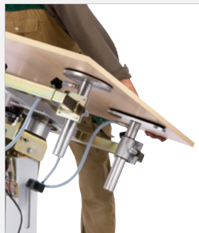
Holding can be turned inside for smaller workpieces
